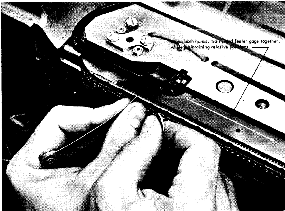
Figure 77. Method of Checking Accumulated Interslug Gap
