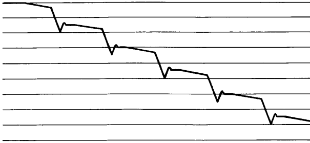
Figure 51. Bypass Adjusted too Tight (Hydraulic Bounce)
