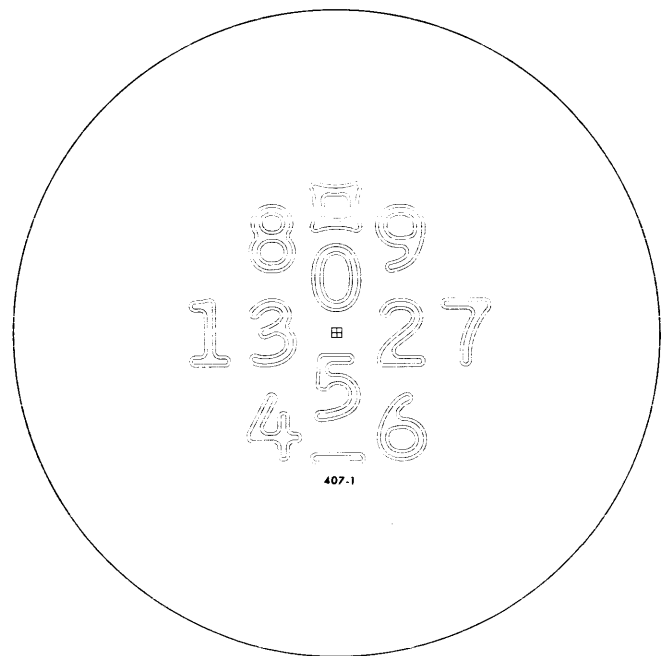
Figure 101. Pocket Comparator 407-1 T-Reticle
